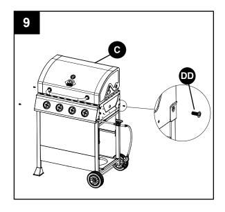
10. Pre-assemble two M6x16 bolts (DD) onto the grill body assembly (C) and do not tighten them and make sure to leave a 5mm gap between the bolt and grill body's end cap. Then hang the left side table assembly (J) on the bolts and fasten the left side table assembly (J) with three M6x16 bolts (DD) and tighten all bolts.
