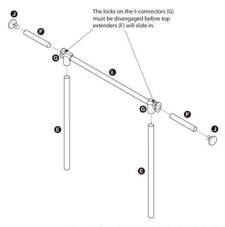
1. End caps (J) ar e designed to fit very tightly into top extenders (F). Apply firm even pressure taking care not to bend or damage top extenders (F) by tapping or hitting.
