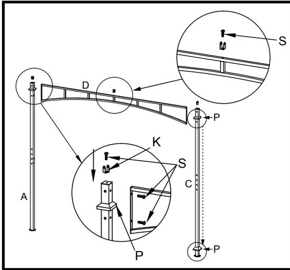
1. Place a Pole Foot (P) through Pole A (A) and slide the Pole Foot (P) down the length of Pole A (A) until it reaches the bottom of the pole. Follow this same procedure with Pole B (B) and both of Pole C (C).
