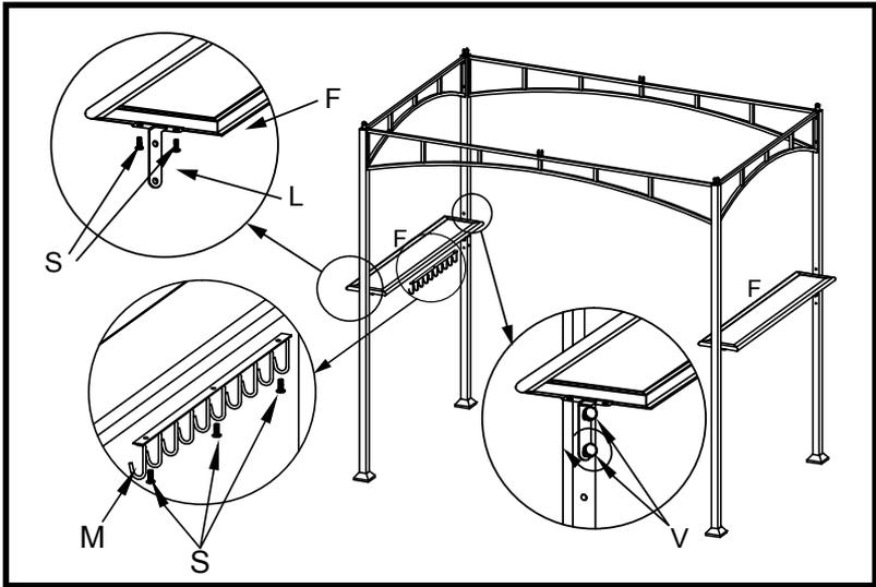
3. Screw in a Shelf Brace (L) onto the bottom of either end of the Shelf (F), using two M6x15mm screws (S). Follow this same step with the second Shelf (F).
