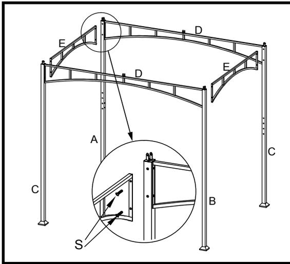
2. Screw in one side of Long Arch (D) into the top of Pole B (B), using two M6x15mm screws (S). Screw in the other side of the same Long Arch (D) into the top of the second Pole C (C), using two M6x15mm screws (S).
