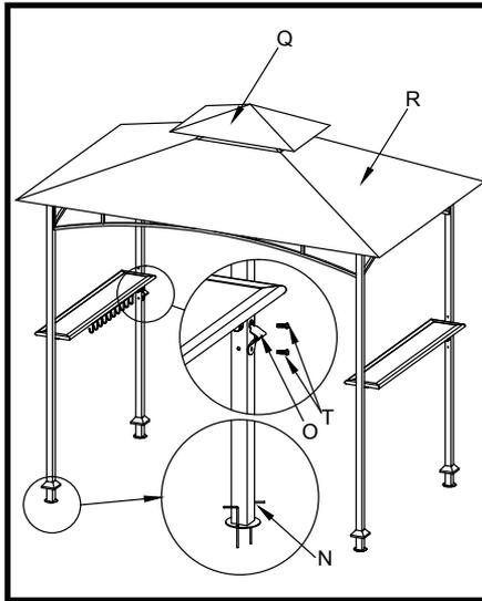
5. Screw in Bottle Opener (O) with the bottle opener hole facing the ground into Pole A (A), underneath the Shelf (F) with Utensil Rack (M) attached to it, using two [white zinc] M6x15mm screws (T). Lift the Pole Foot (P) up from each pole and insert a Stake (N) through the holes at the bottoms of those poles. Place each Pole Foot (P) back in its place covering the Stakes (N).
