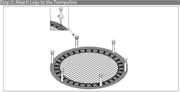
Locate the small cardboard box with the six Trampoline Legs. Twist a leg onto the threaded grooves on each Leg Base post. Do not overtighten.
